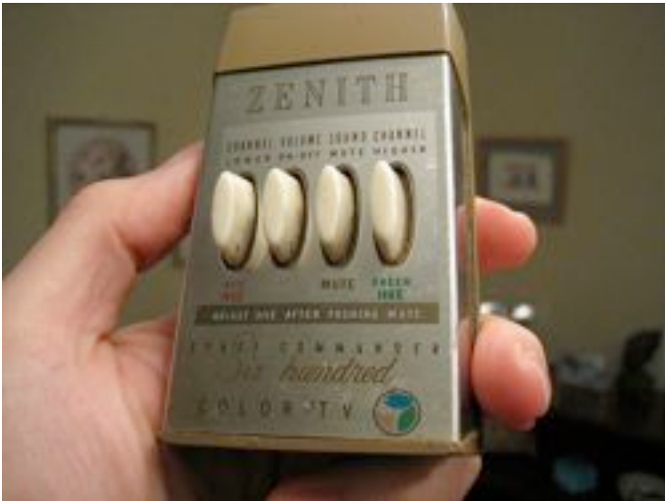
Figure 1.4 Although there had been remote-control planes and boats previously (mostly for military use), the Space Commander television remote removed proximity from control for consumers.
